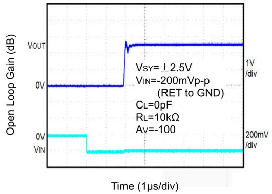
**Figure 2-10 Negative Overvoltage Recovery**
