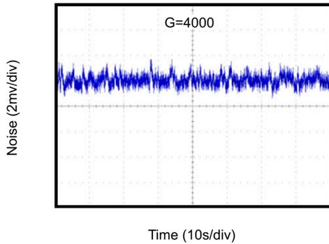
**Figure 2-11 0.1Hz to 10Hz Noise at +5V**
