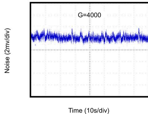
**Figure 2-12 0.1Hz to 10Hz Noise at +2.5V**
