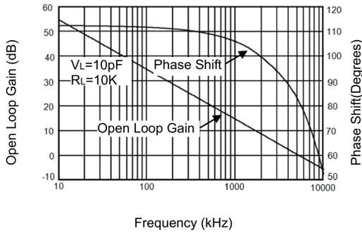
**Figure 2-7 Open Loop Gain, Phase Shift vs. Frequency at +5V**
