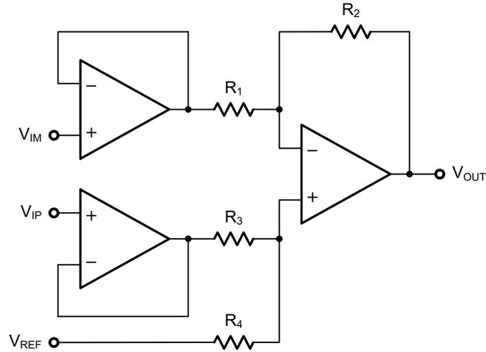
Figure 4-3 Instrument Amplifier
