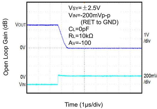
**Figure 2-9 Positive Overvoltage Recovery**
