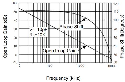
**Figure 2-8 Open Loop Gain, Phase Shift vs. Frequency at +2.5V**
