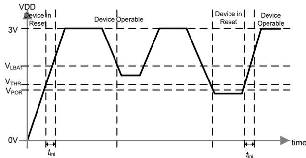
Figure 5-2 Power-On and Under-Voltage Reset Behavior
