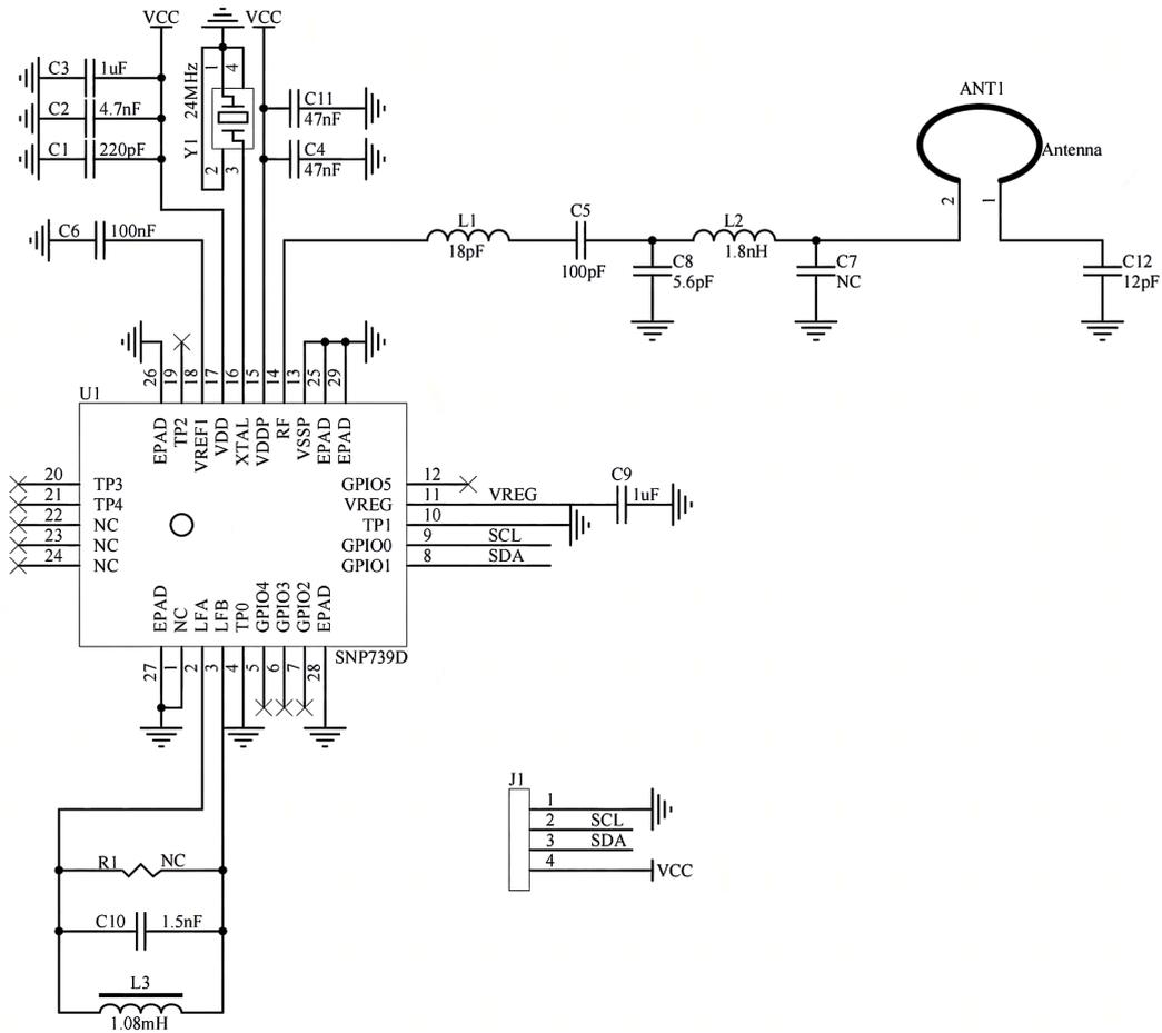
Figure 6-1 Application Circuit
