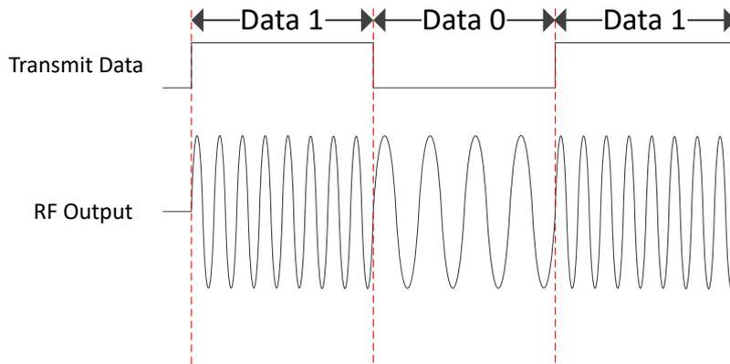
Figure 5-9 FSK modulation
