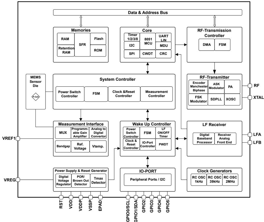
Figure 5-1 Block Diagram
